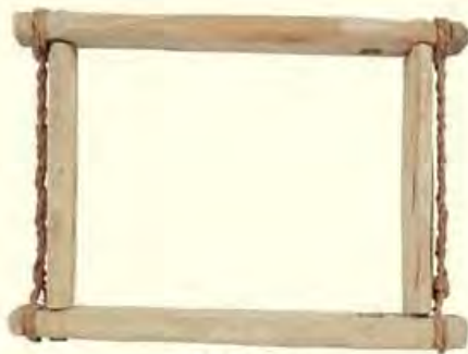
"Milban" (a wooden frame for moulding mud bricks)
