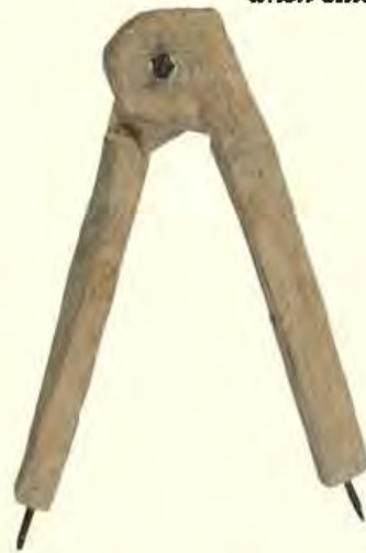
"Firjar" (compasses for measuring when cutting wood)
